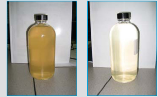
Chilled Water Before and After
