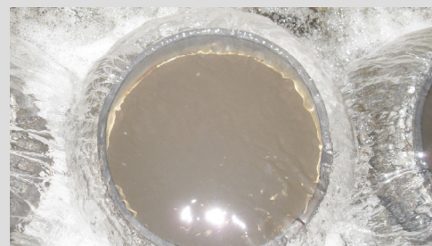
Good Suspended Solids Removal
